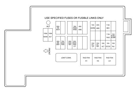
The high-current fuses are coded as follows.
